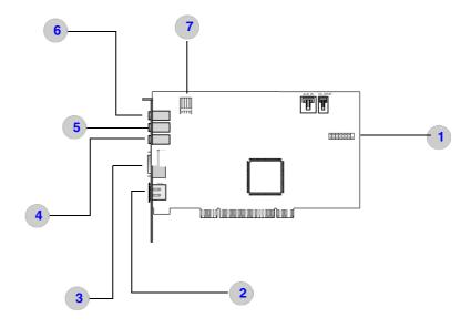
*Figure 1-2:* Jacks, connectors and ports
